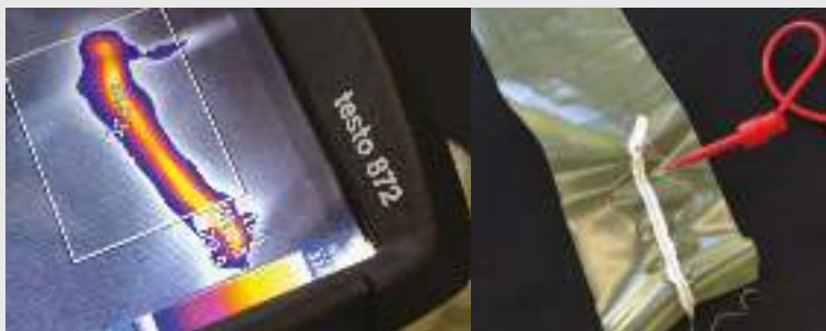
Figure 23. Comparative study showing the effects of exposed con- ductive yarn and the heat emitted from the source: Eurecat, Bar- celona.
