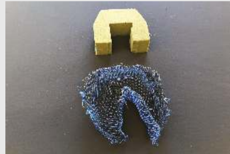
Figure 11. Early Examination of Material Composition for its Deformation using Heat: Polypropylene and Nylon Monofilament: Eurecat, Barcelona.
